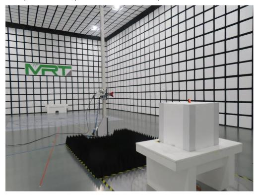
Description: Radiated Spurious Emissions Test Setup for above 1GHz (Zoom Photo)
