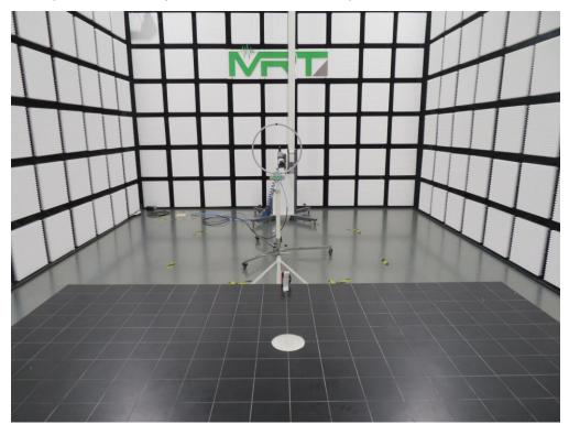
Description: Radiated Spurious Emissions Test Setup for 30MHz ~ 1GHz
