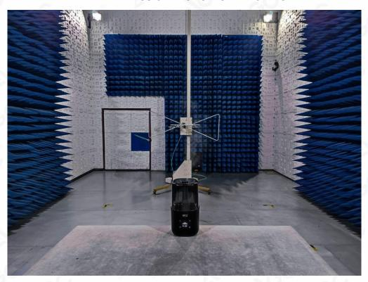
RADIATED EMISSION TEST SETUP ABOVE 1GHz
