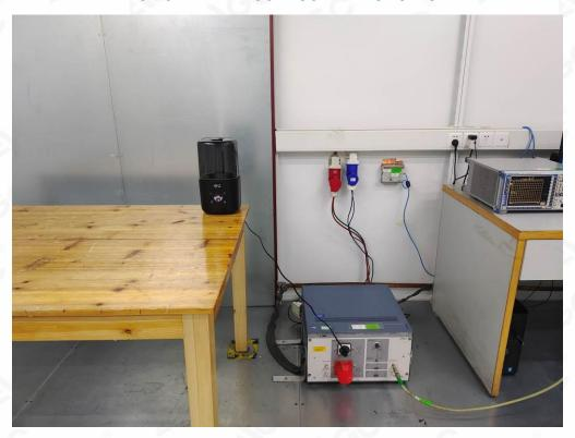
RF CONDUCTED TEST SETUP
