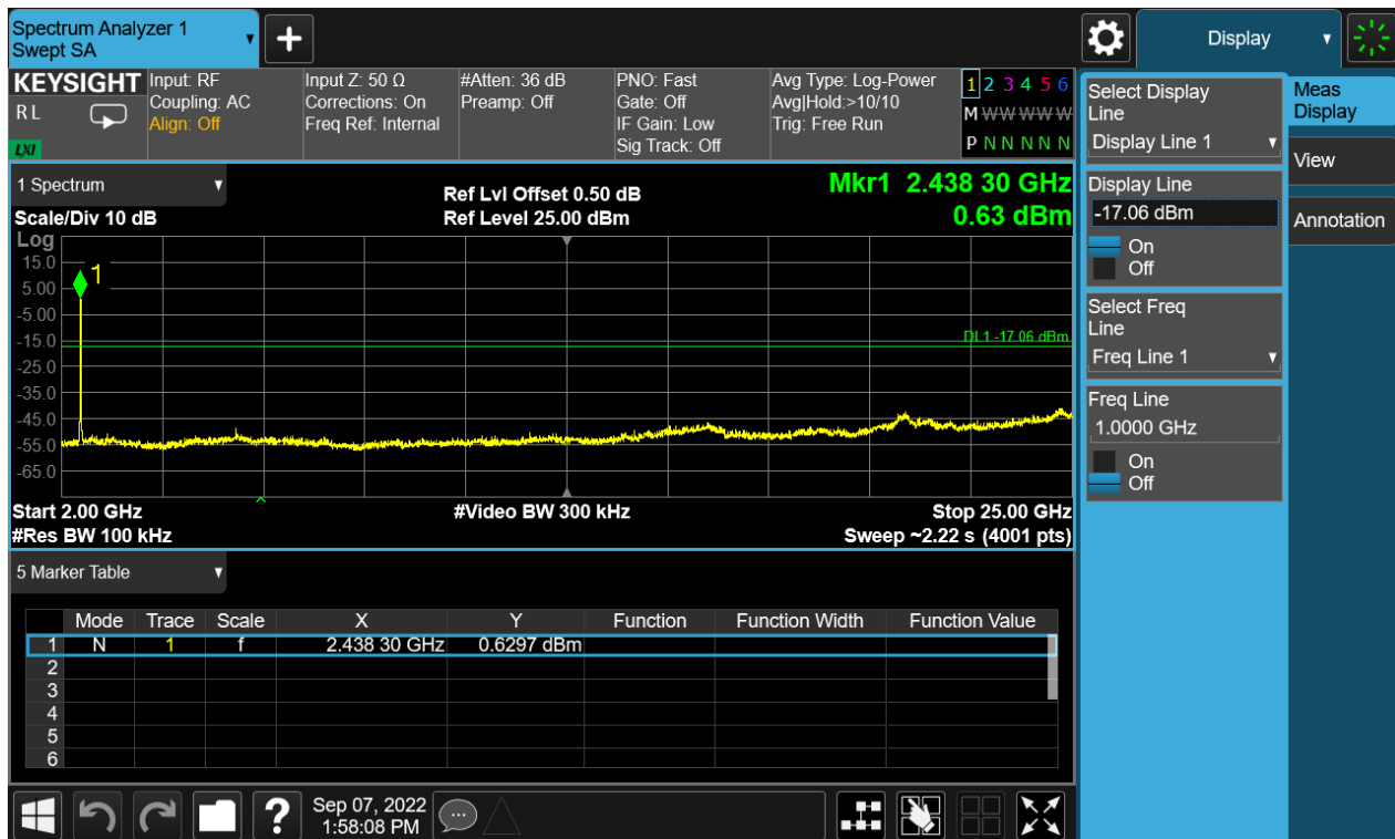
Figure 78: The plots of Conducted Spurious Emission & Authorized-band band-edge, 802.11n(HT20), 2462MHz Carrier Level
