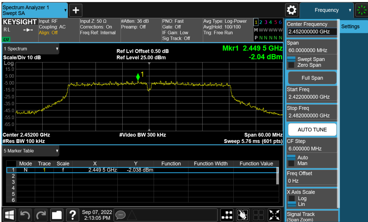
Figure 90: The plots of Conducted Spurious Emission & Authorized-band band-edge, 802.11n(HT40), 2452MHz Band Edge
