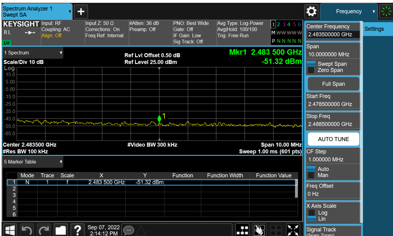
Figure 90: The plots of Conducted Spurious Emission & Authorized-band band-edge, 802.11n(HT40), 2452MHz Band Edge
