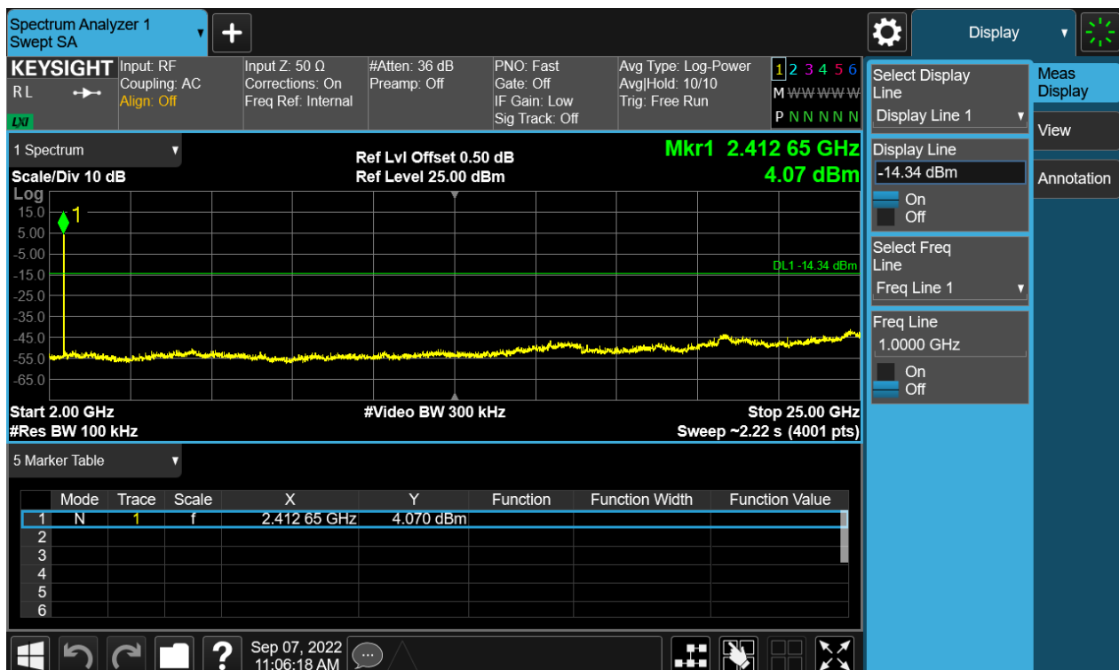
Figure 52: The plots of Conducted Spurious Emission & Authorized-band band-edge, 802.11b, 2412MHz Conducted spurious emissions 2GHz-25GHz
