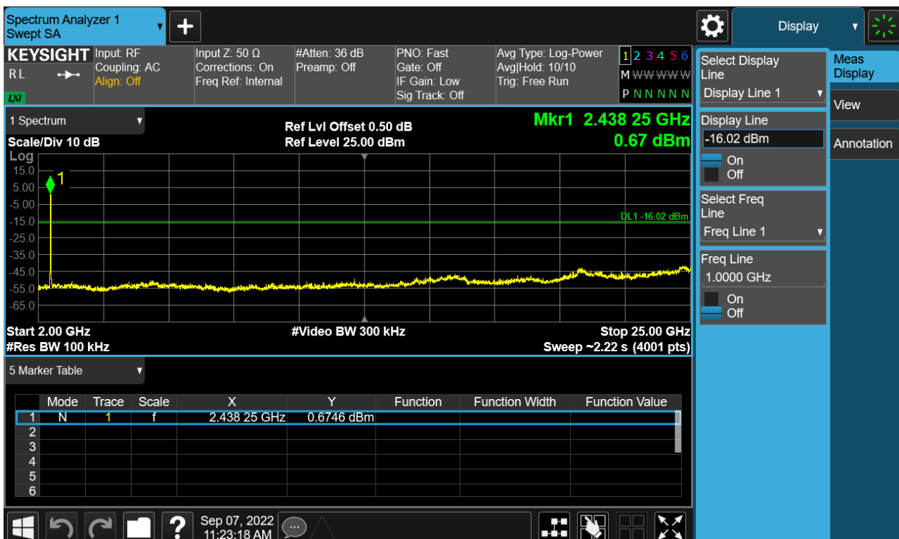
Figure 66: The plots of Conducted Spurious Emission & Authorized-band band-edge, 802.11g, 2437MHz Conducted spurious emissions 2GHz-25GHz
