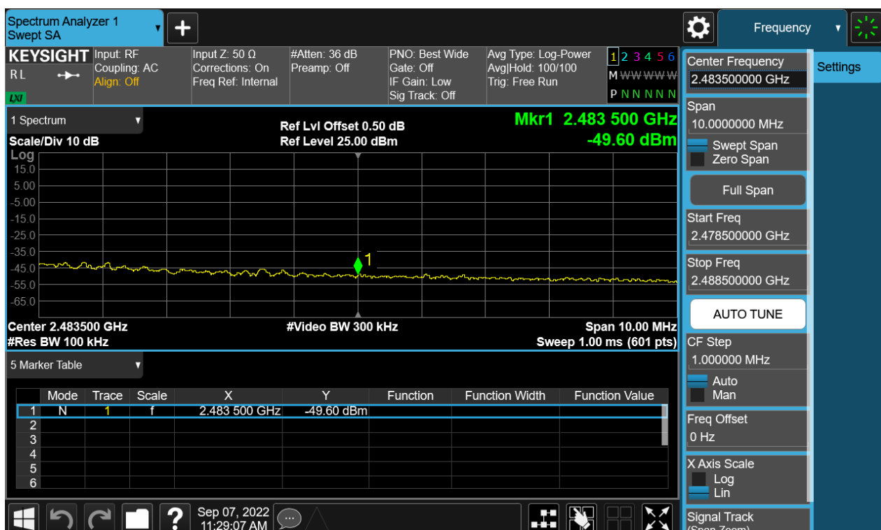
Figure 68: The plots of Conducted Spurious Emission & Authorized-band band-edge, 802.11g, 2462MHz Band Edge
