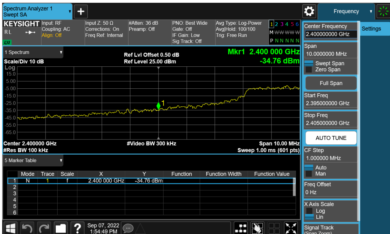
Figure 13: The plots of Conducted Spurious Emission & Authorized-band band-edge, 802.11n(HT20), 2412MHz Band Edge
