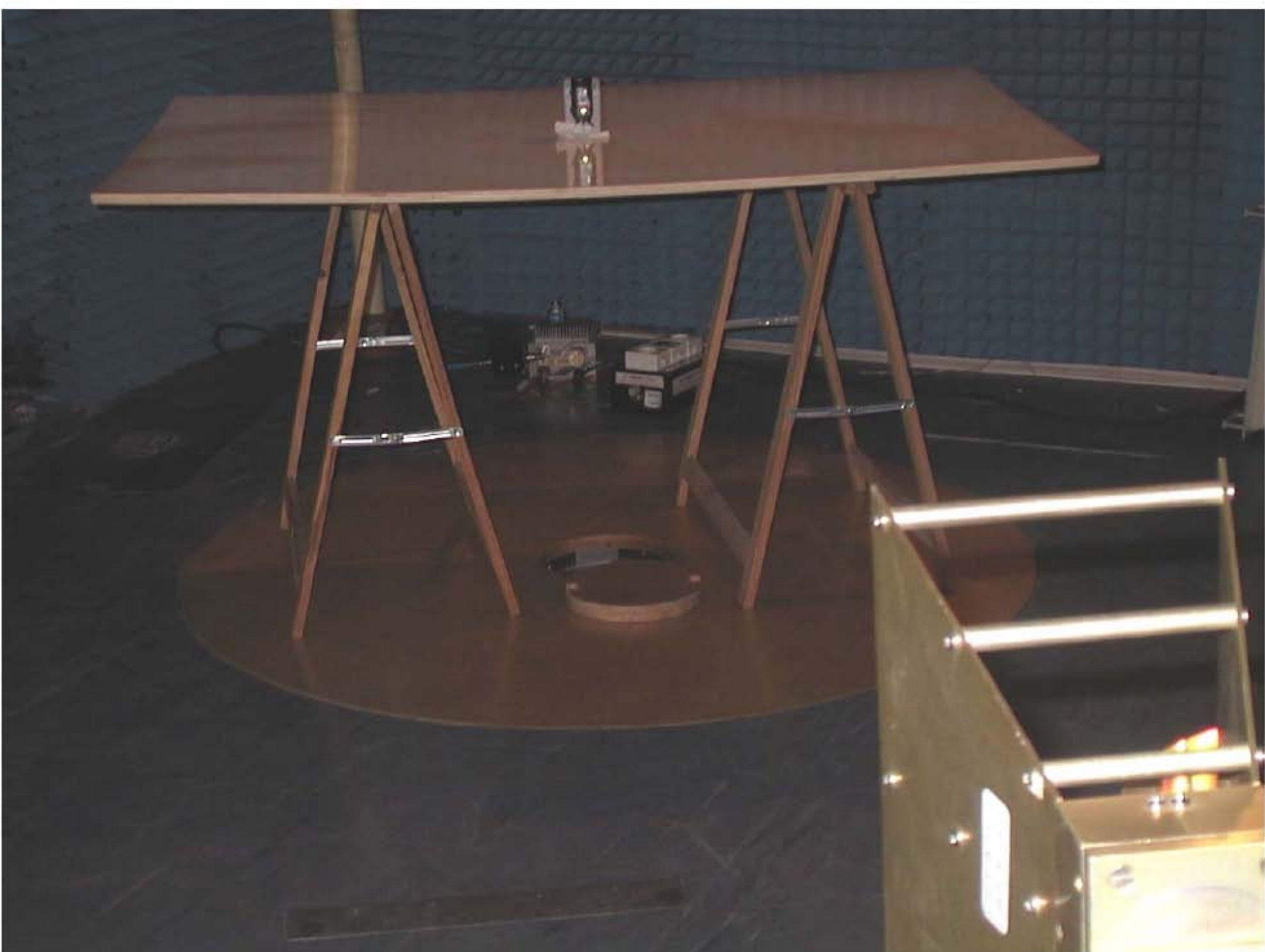
Photograph-4 Set up for Radiated Emission 1GHz-5GHz
