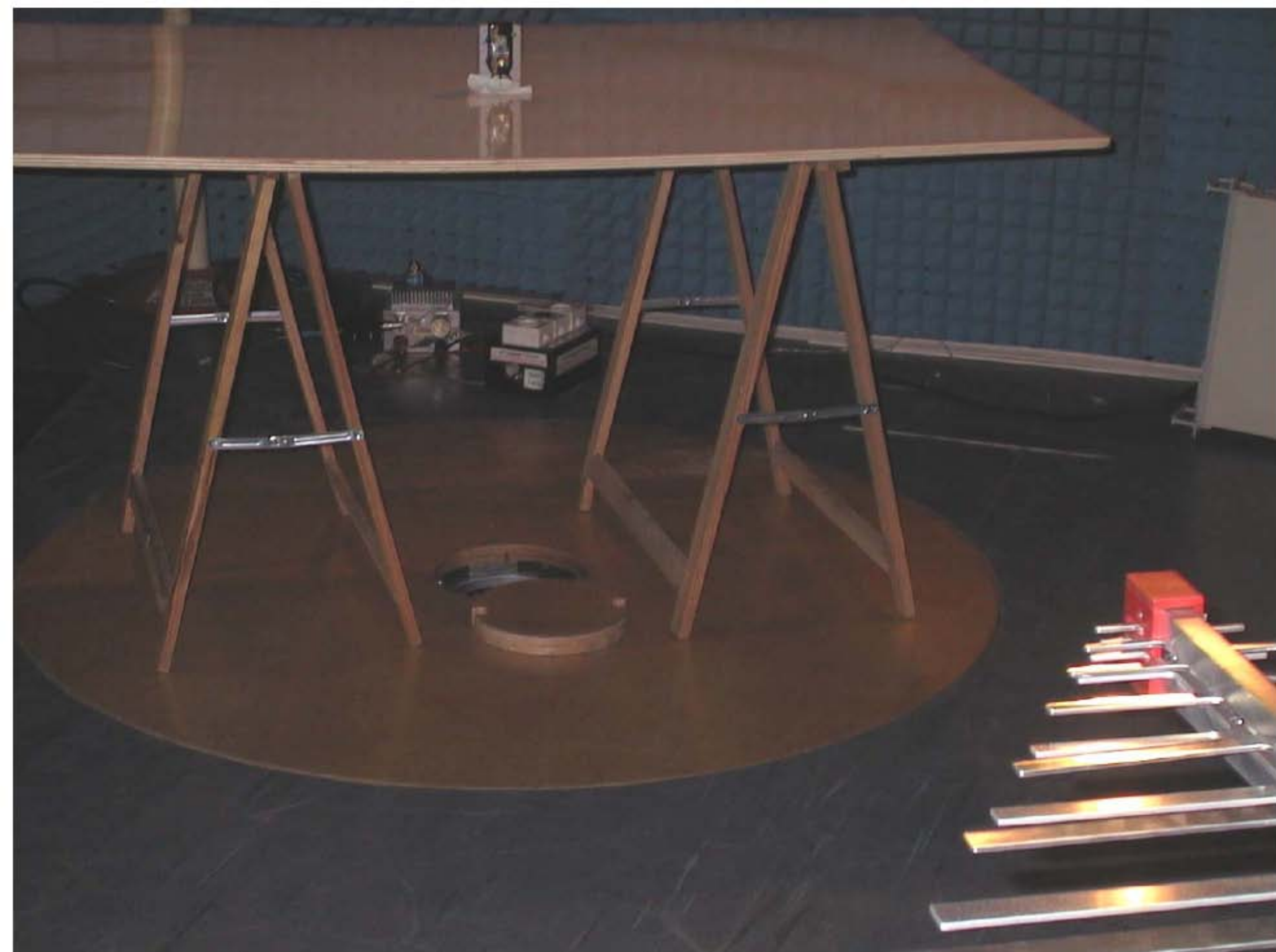
Photograph-3 Set up for Radiated Emission 30MHz-1GHz
