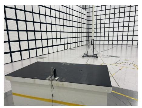
3. Radiated Emission setup photo (Above 1 GHz~18 GHz)
