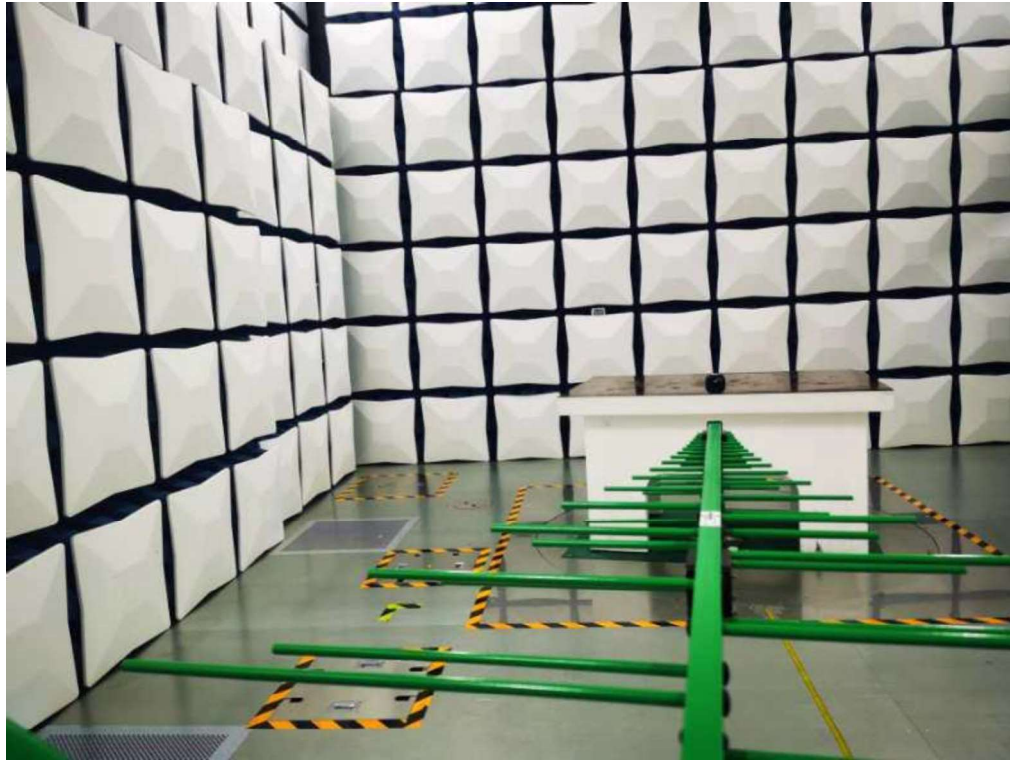
Photograph 2: Set-up for Radiated Emission, above 1GHz
