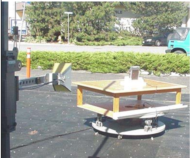
Photograph B.7-2 - Horn Receive Antenna with DUT Antenna - DUT "Portrait" Configuration
