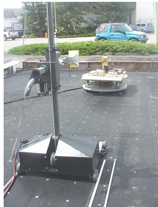
Photograph B.7-4 - Horn Substitution Setup
