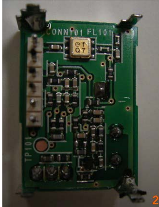
Tuner – Rear with shield
