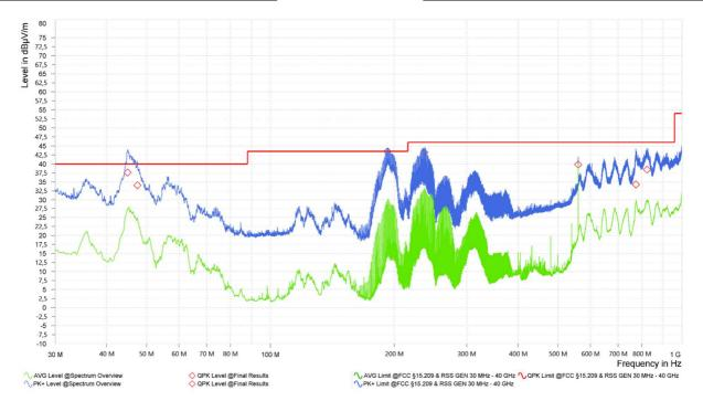
The results of the standard subsequent measurement in a semi-anechoic chamber are indicated in the table below. The limits as well as the measured results (levels) refer to the above-mentioned standard while taking account of the specified requirements for a 3 m measuring distance.
