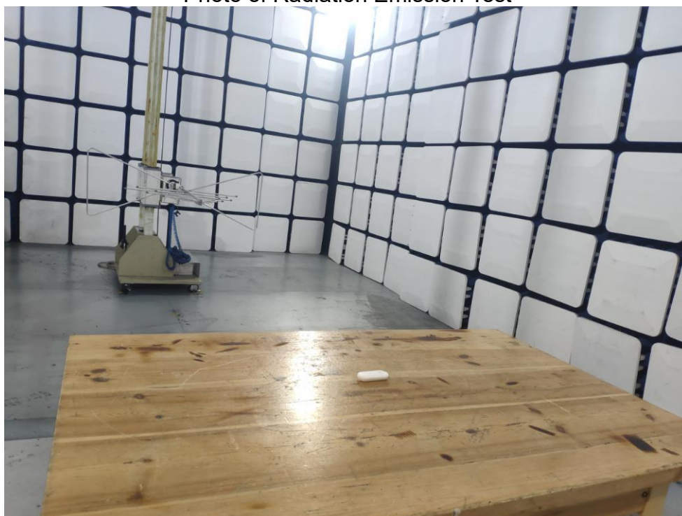
FCC ID: 2APSE-CLIMATE2 Photo of Radiation Emission Test
