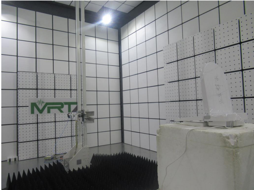
Description: Radiated Spurious Emission Test Setup for 18~40 GHz
