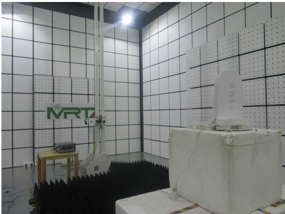
Description: Radiated Spurious Emission Test Setup for 18~40 GHz
