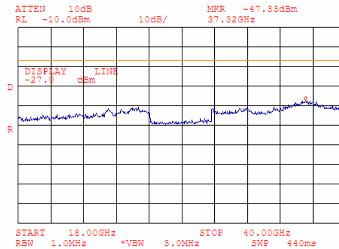
Plot 9.1.41 Conducted emission measurements from 18 to 40 GHz at the 5.785GHz carrier frequency
