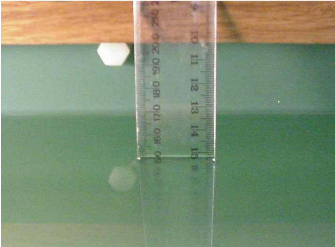
Photo of liquid Depth in Flat Phantom
