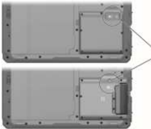
Battery Hot Swapping Indicator
