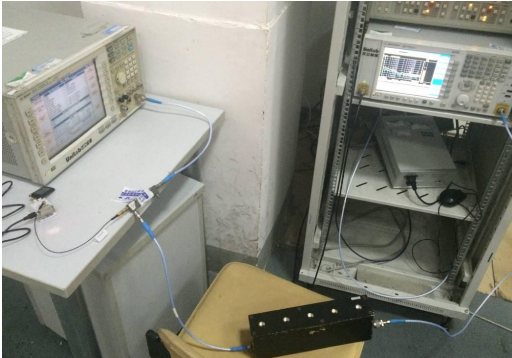
Frequency Stability Under Temperature & Voltage Variations Setup
