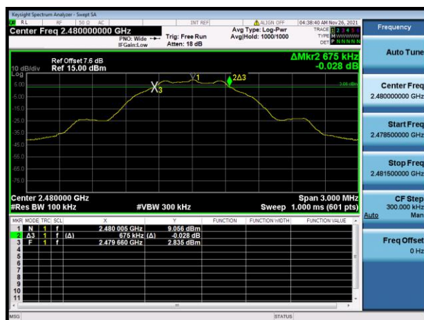
GFSK (BLE 1Mbps) HIGH CHANNEL
