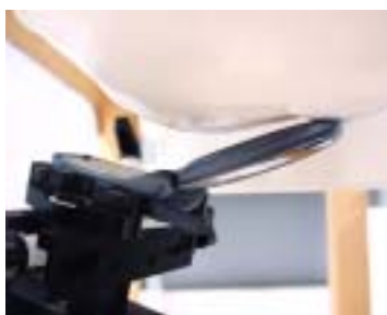
Figure 8.9 Left Head SAR Test Setup -- Ear/Tilt 15° Position--
