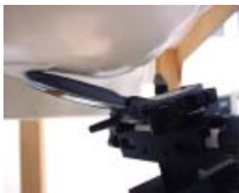
Figure 8.3 Right Head SAR Test Setup -- Ear / Tilt 15° Position --
