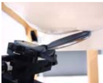
Figure 8.5 Left Head SAR Test Setup -- Ear / Tilt 15° Position --
