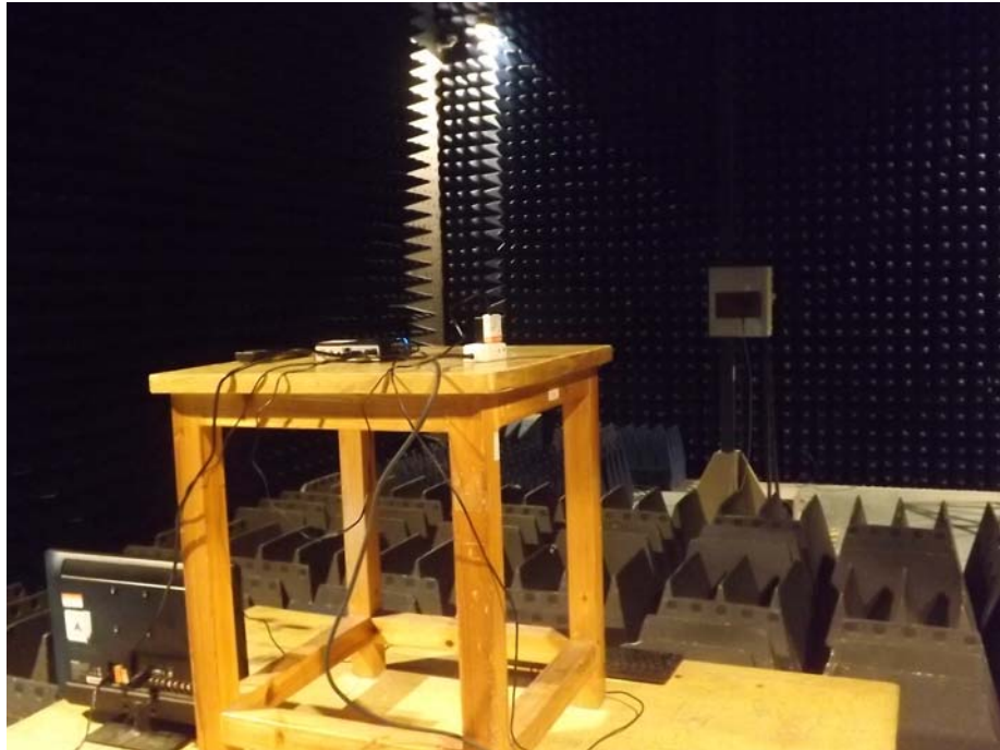
14.2 Photograph – Conducted Emission Test Setup at Test Site 2#
