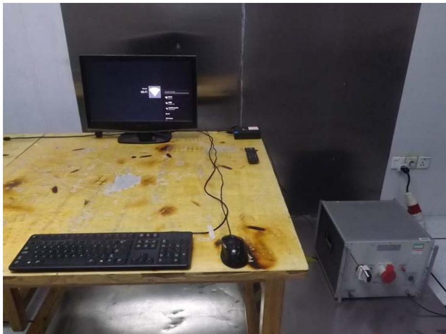
14.2 Photograph – Conducted Emission Test Setup at Test Site 2#
