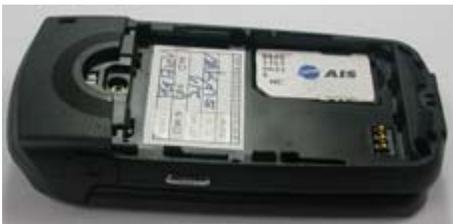
3. If you want to remove the SIM card, push the SIM card to the arrow direction as shown in the below figure.
