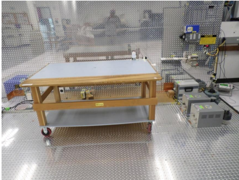
Figure 5: Conducted Emissions Limits, Terminal, Test Setup, Front View
