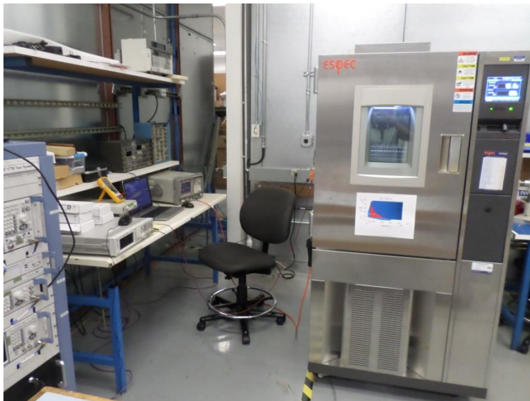
Figure 12: Frequency Stability, Terminal, Test Setup
