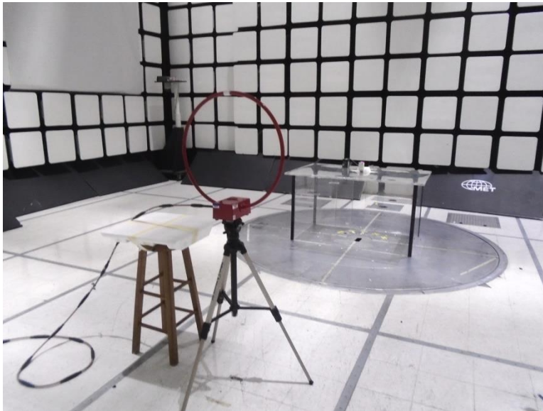
Figure 9: Radiated Spurious Emissions, 0.009 MHz – 30 MHz, Test Setup
