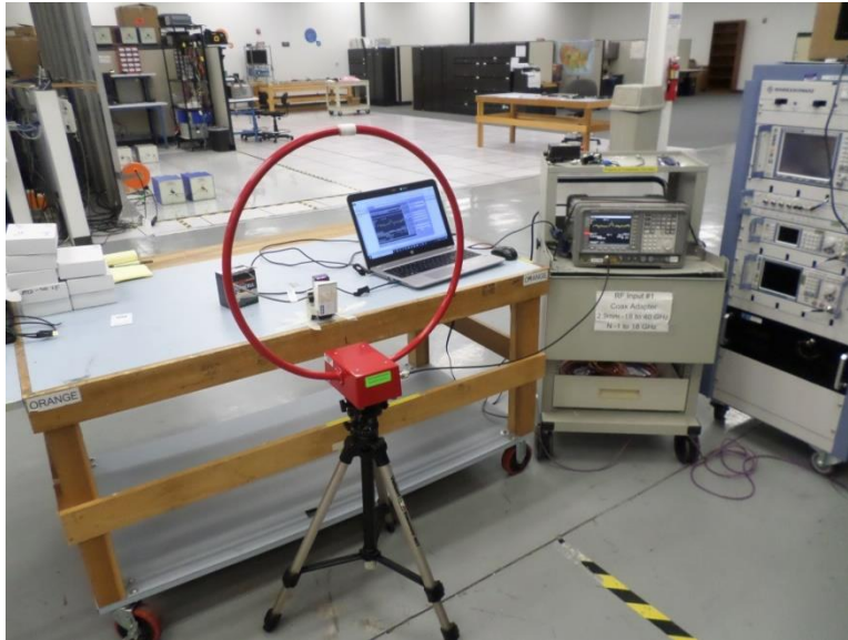
Figure 7: 20 dB Occupied Bandwidth, Pigtail, Test Setup
