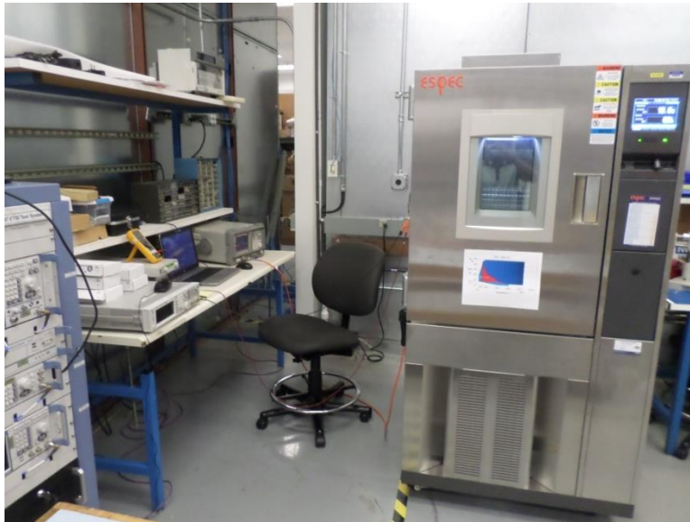
Figure 11: Frequency Stability, Pigtail, Test Setup
