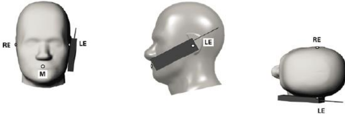
Fig. 11.3 Illustration for Cheek Position
