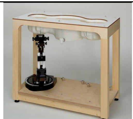
Fig. 8.7 Photo of SAM Twin Phantom
