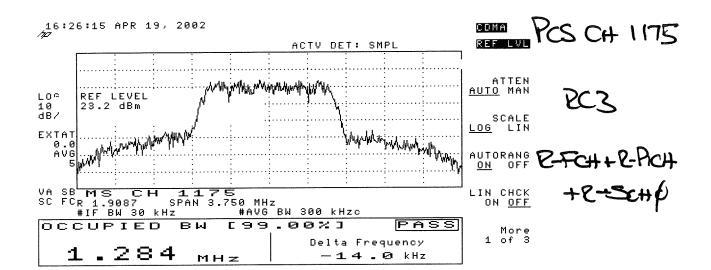
RC3 R-FCH and RC3 R-FCH+R-SCH Spurious Up to 10<sup>th</sup> Harrnonics
