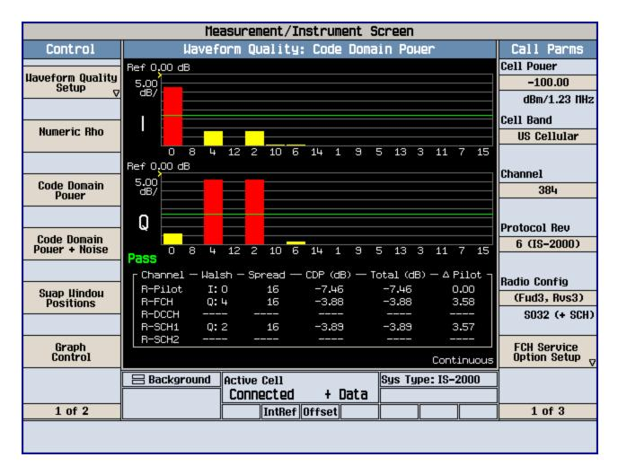
The plots of occupied bandwidth and spurious emission for CDMA cellular, ch384 are attached in the proceeding pages.
