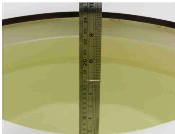
Fig 11.1 Photo of Liquid Height for Body SAR
