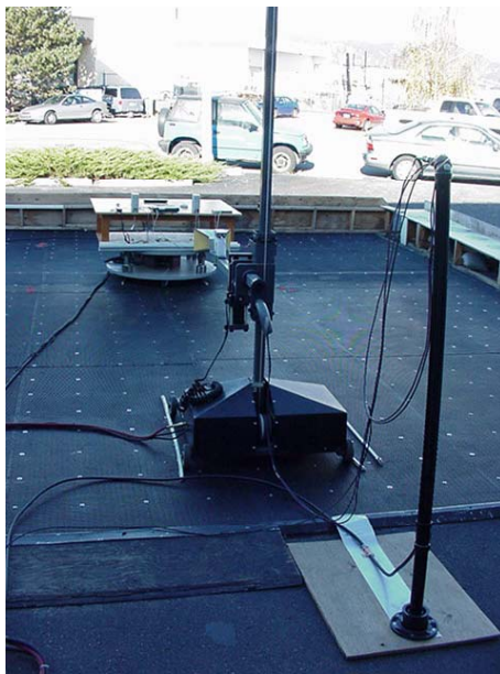
Photograph J.7-3 - Portable 3 m Horn setup
