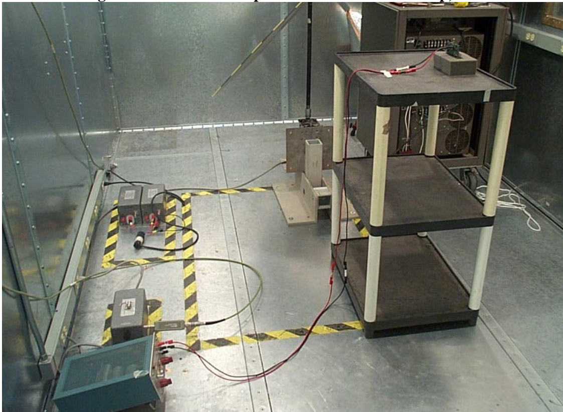
Figure C – 2 AC Conducted Emissions Test Setup
