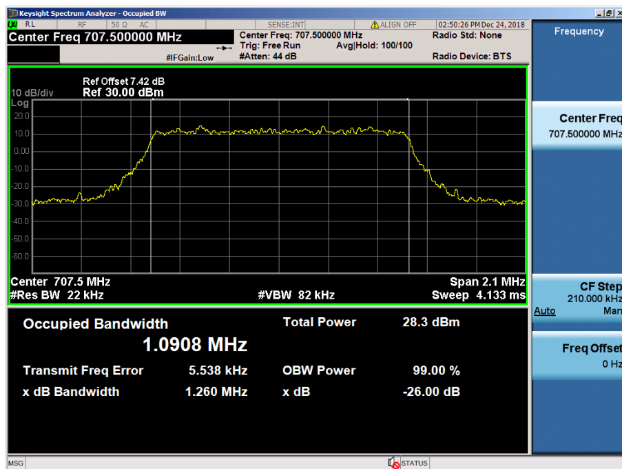
LTE Band 12 / 1.4 MHz / 16QAM - RB Size 6
