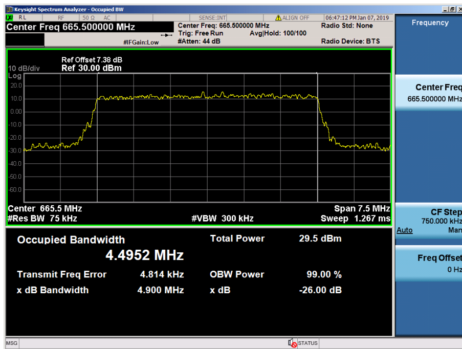
LTE Band 71 / 5 MHz / QPSK - RB Size 25
