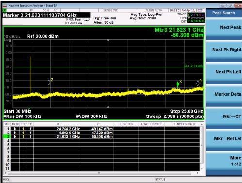
Note: The peak emissions without marker on the above plots are fundamental wave and need not to compare with the limit. The GFSK modulation is the worst case and only those data recorded in the report.
