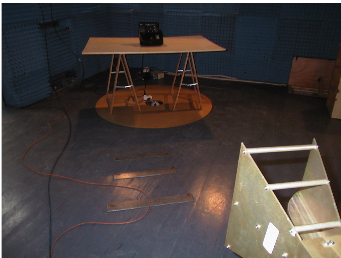
Photograph/ 2 Radiated Emission 1-2GHz test setup
