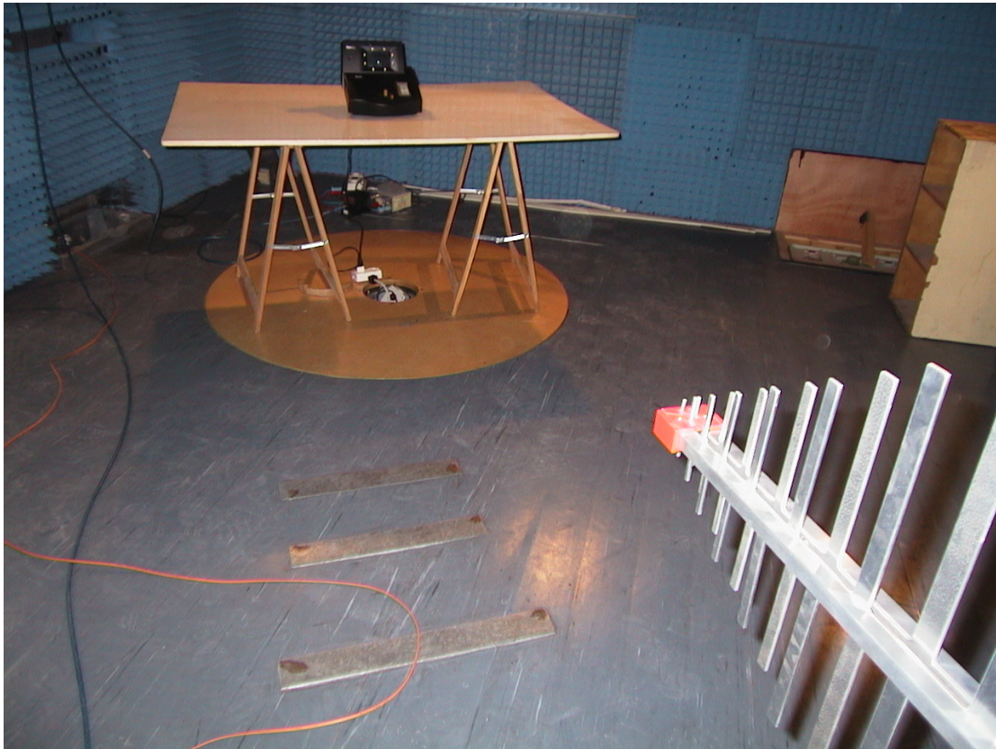
Photograph/ 1 Radiated Emission 30-1000MHz test setup
