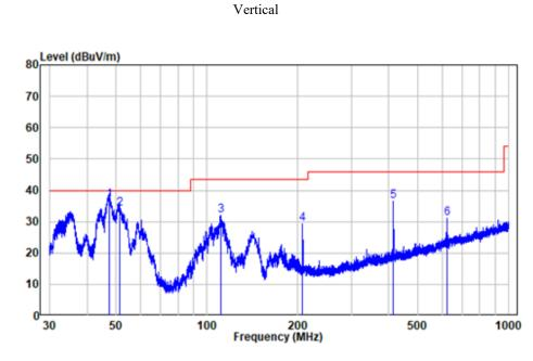
Site : chamber Condition: 3m VERTICAL Job No. : SZNS220607-24962E-RF Test Mode: FP Adapter : VT05UUS06040
