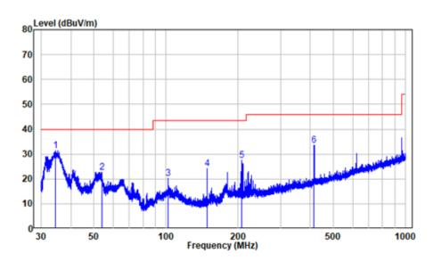
Site : chamber Condition: 3m VERTICAL Job No. : SZNS220607-24962E-RF Test Mode: FP Adapter : S003AKU0600040
