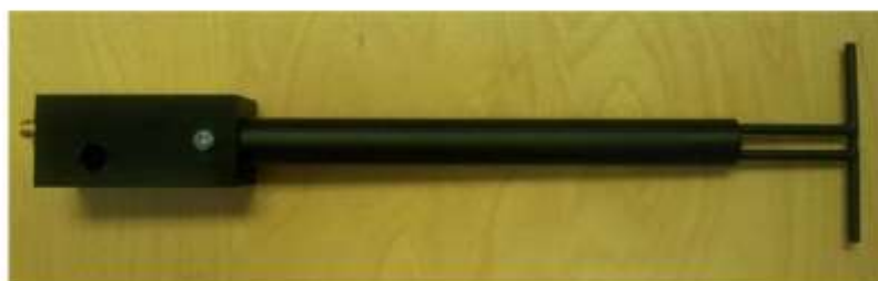
Figure 1 – MVG COMOSAR Validation Dipole
