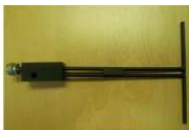
Figure 1 – MVG COMOSAR Validation Dipole
