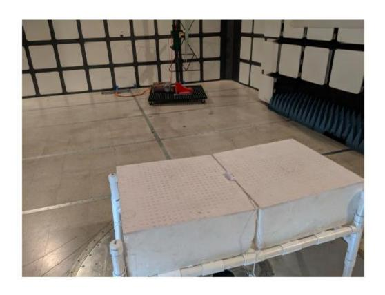
NORTEK SECURITY & CONTROL LLC FLOOD AND TEMPERATURE DETECTOR MODEL: 2GIG-FT1e-345 FCC SUBPART C - RADIATED EMISSIONS < 1GHZ
