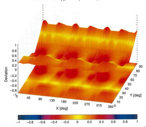
Probe isotropy for E<sub>tot</sub>: probe rotated  $\phi=0^\circ$  to 360°, tilted from field propagation direction  $\vec{k}$  Parallel to the field propagation ( $\psi=0^\circ-90^\circ$ ) at 30 GHz: deviation within  $\pm 0.38$  dB Parallel to the field propagation ( $\psi=0^\circ-90^\circ$ ) at 60 GHz: deviation within  $\pm 0.41$  dB
