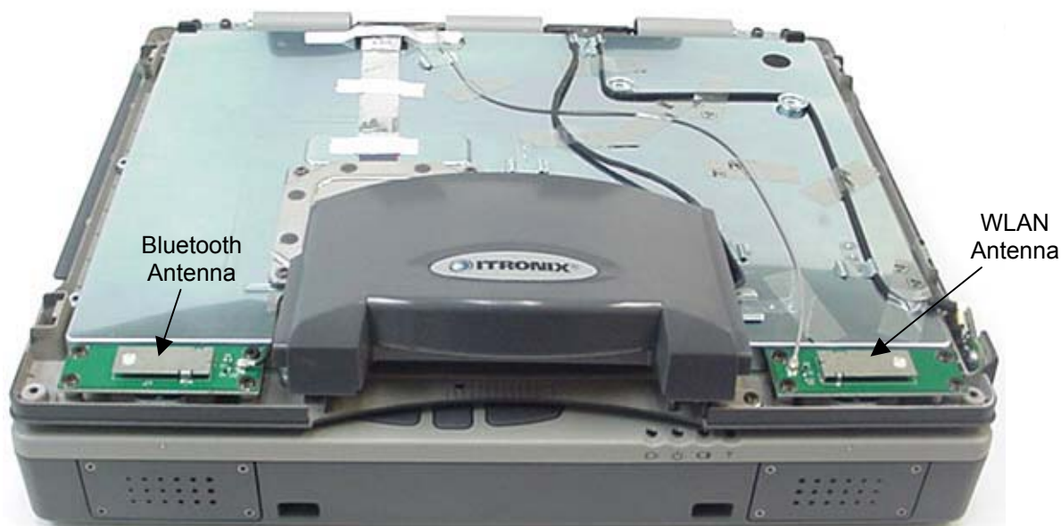
Photograph A-7 - Surface Mount Antenna Placement
