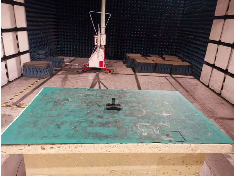
Spurious Emission Test Setup (Below 1GHz)
