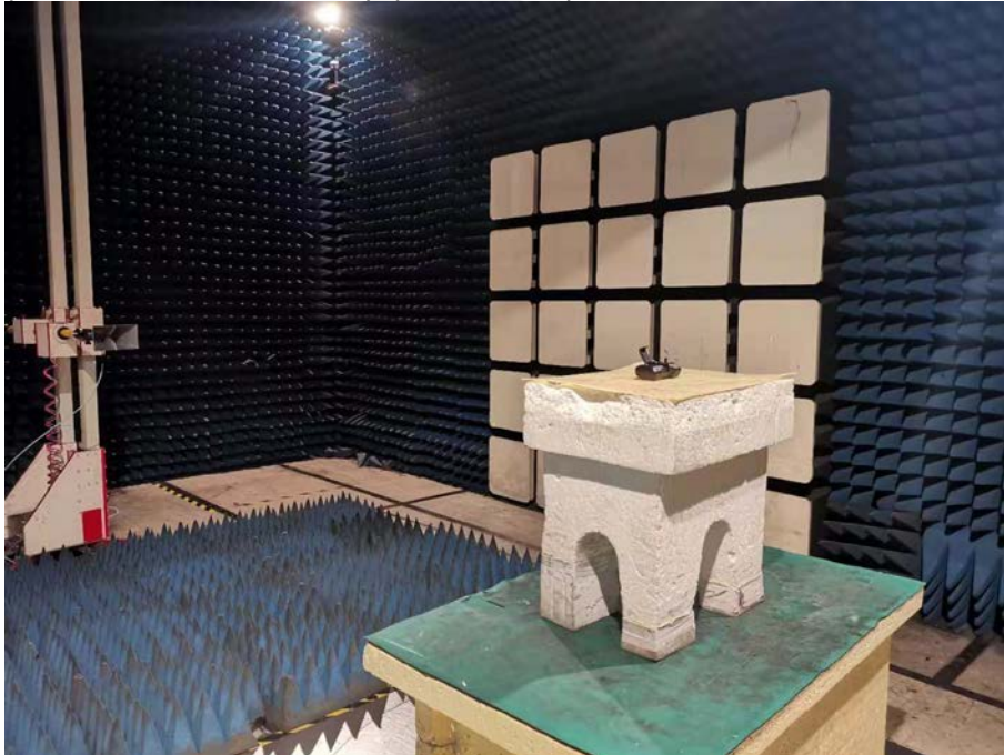
Spurious Emission Test Setup (Above 1GHz)
