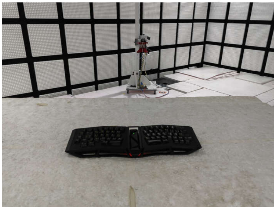
Radiated spurious emission Test Setup-2(Above 1GHz)
