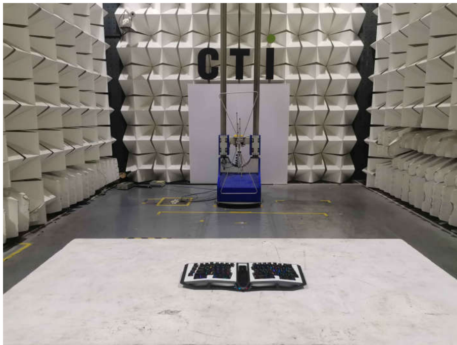
Radiated spurious emission Test Setup-1(Below 1GHz)
