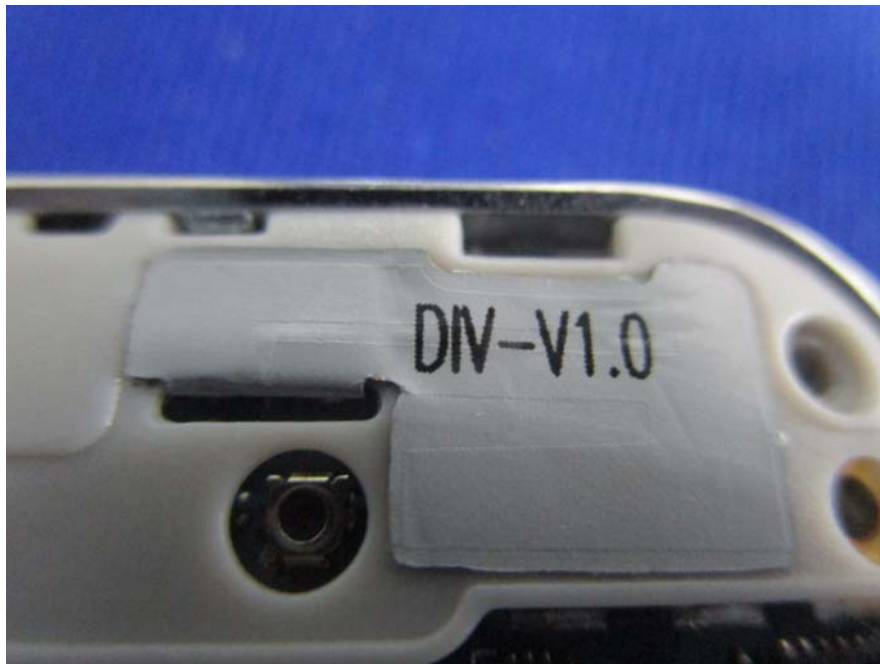
EUT – BT&Wifi Antenna View
