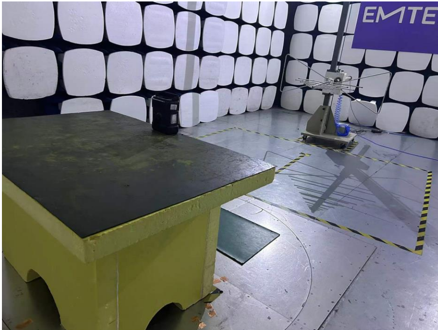
Spurious Emission Test Setup (Below 1GHz)
