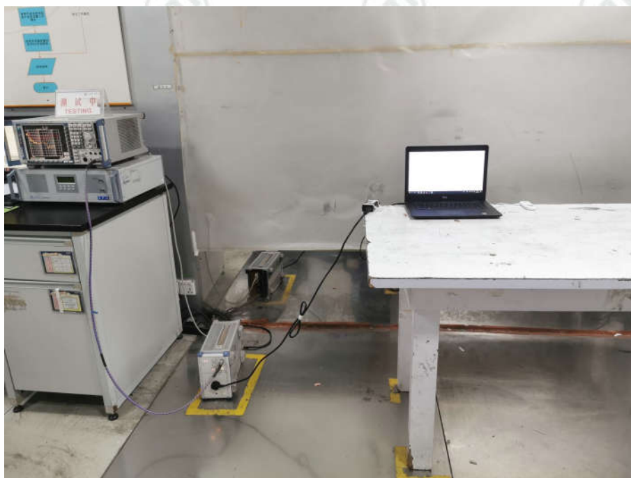
Conducted Emissions Test Setup
