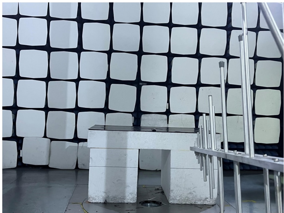
Radiation Emission Test Setup (30MHz to 1GHz)
