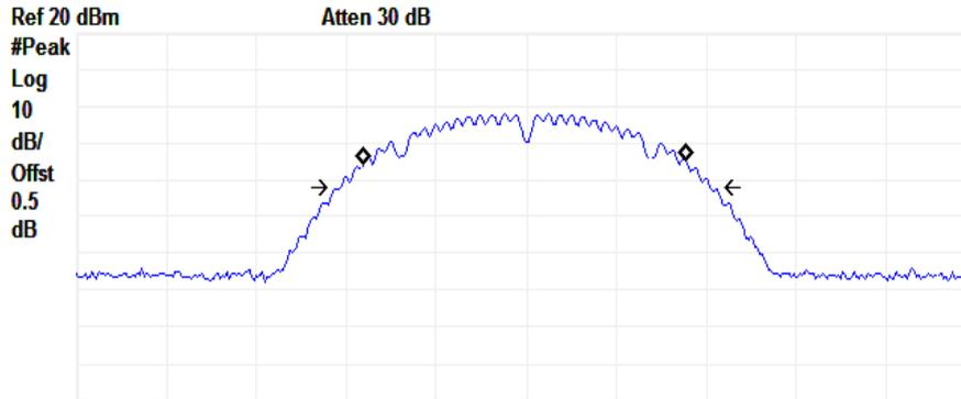
Center 2.437 GHz Span 40 MHz
