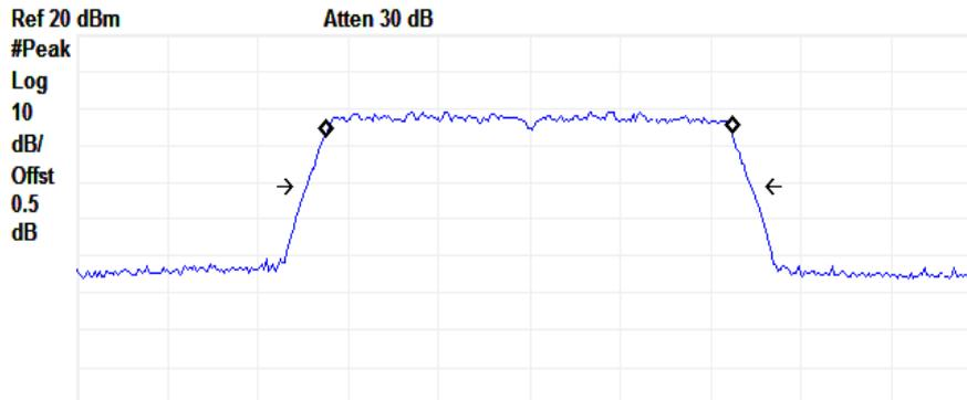
Center 2.437 GHz Span 40 MHz
