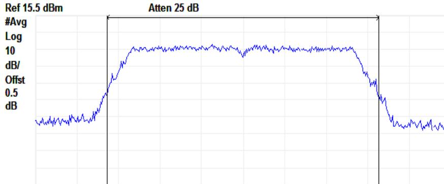
Center 2.437 GHz Span 30 MHz
