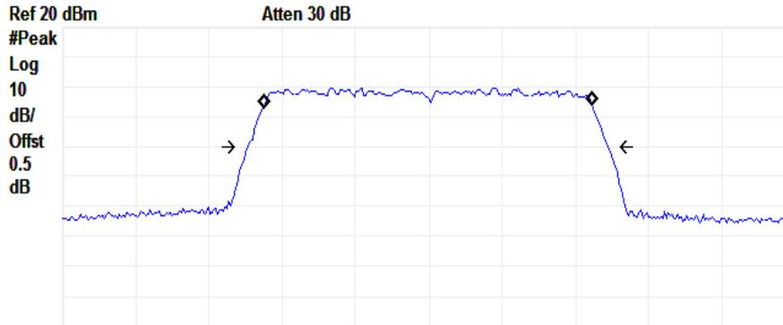
Center 2.412 GHz Span 40 MHz
