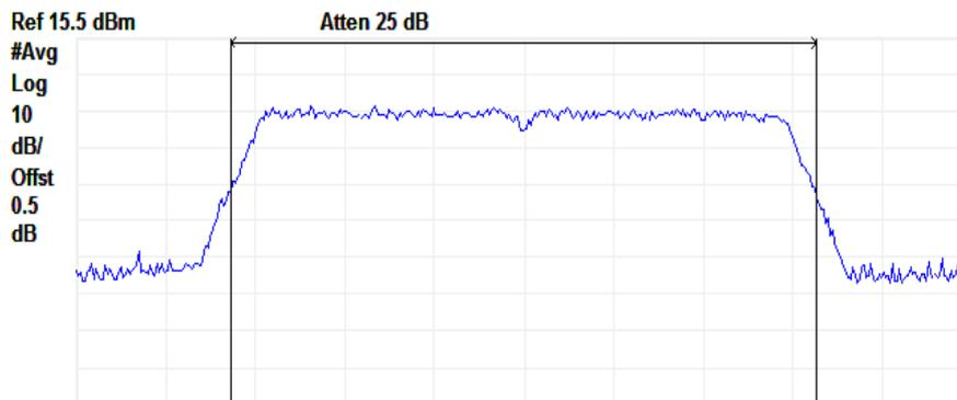
Center 2.437 GHz Span 30 MHz
