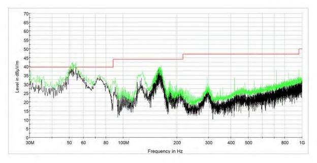
Radiated Spurious Emissions: 30 MHz to 1000 MHz - Horizontal
