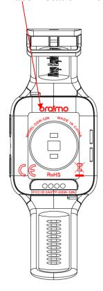
The label shown shall be permanently affixed at a conspicuous location on the device and be readily visible to the user at the time purchase (Labeling requirements per 2.925)
