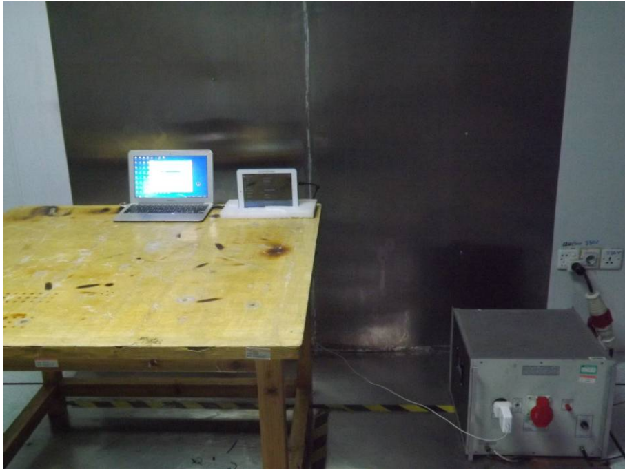
Photograph – Conducted Emission Test Setup at Test Site 2#
