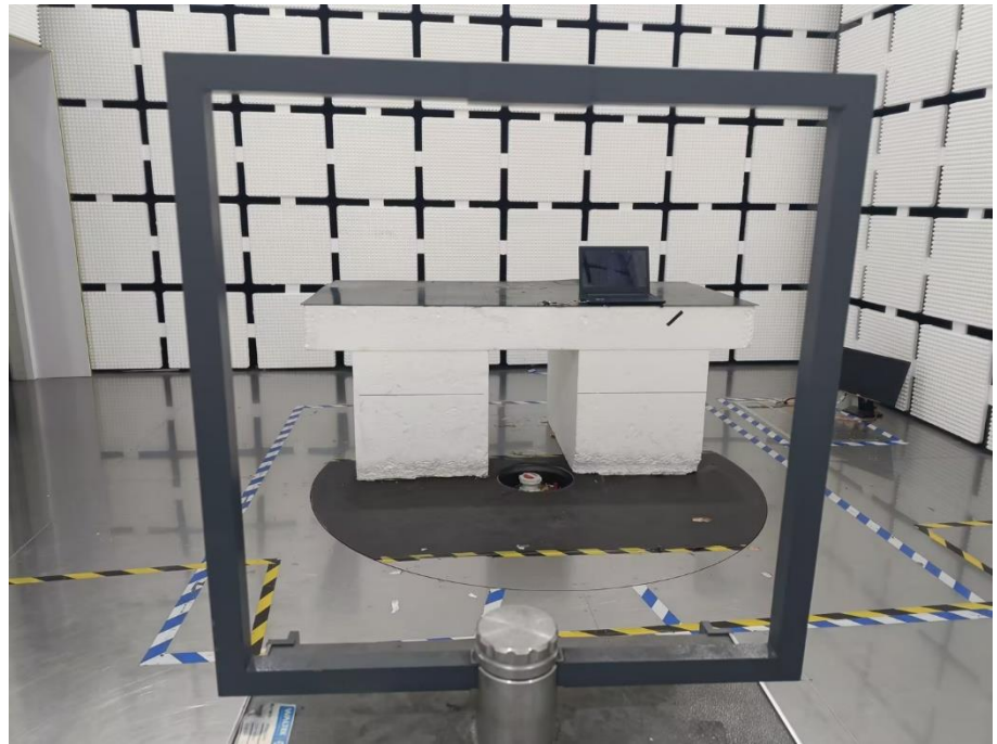
Radiation Emission Test Setup (Below 30MHz)
