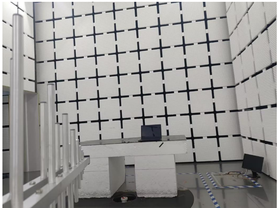
Radiation Emission Test Setup (30MHz to 1GHz)
