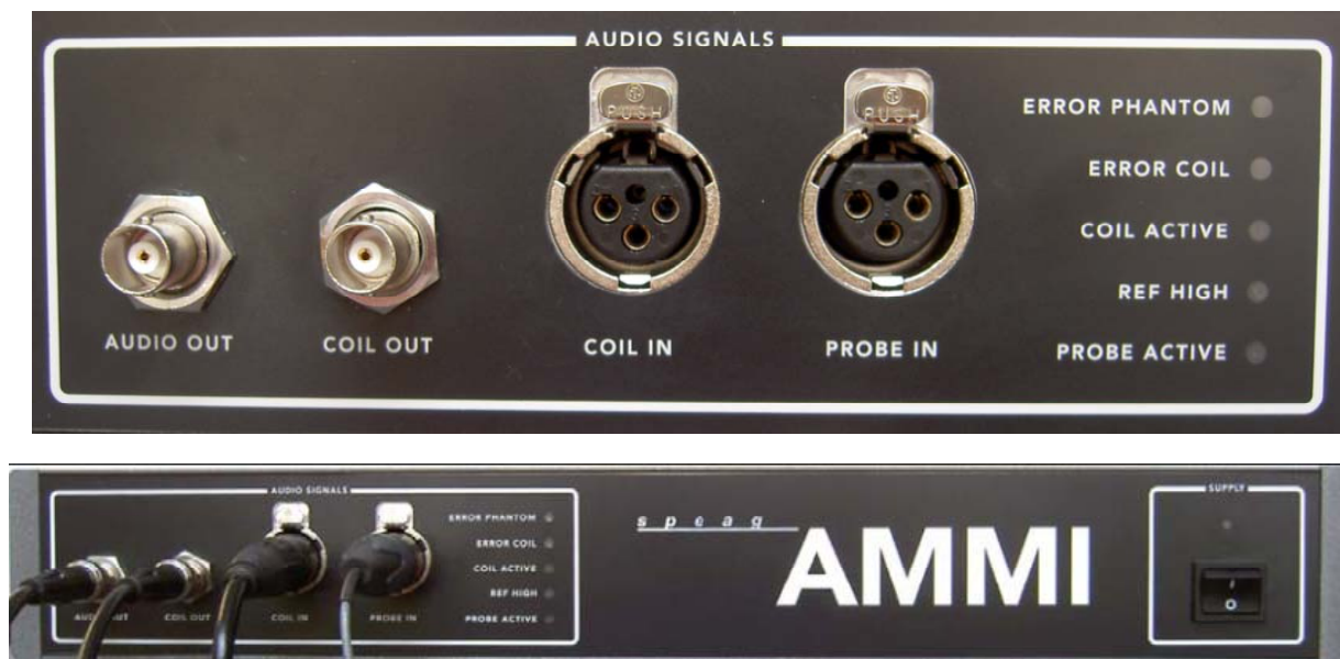
Figure 4 AMMI front panel
