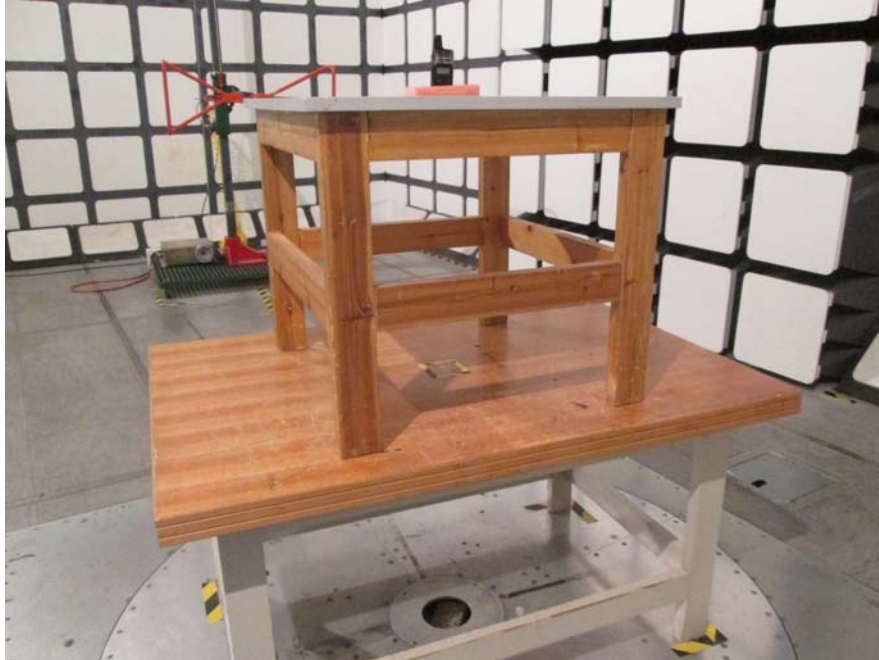
Transmitting Radiated Emissions View (Below 1 GHz)
