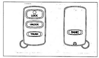
You can control door lock/unlock, trunk opener and panic alarm with the TRANSMITTER.
