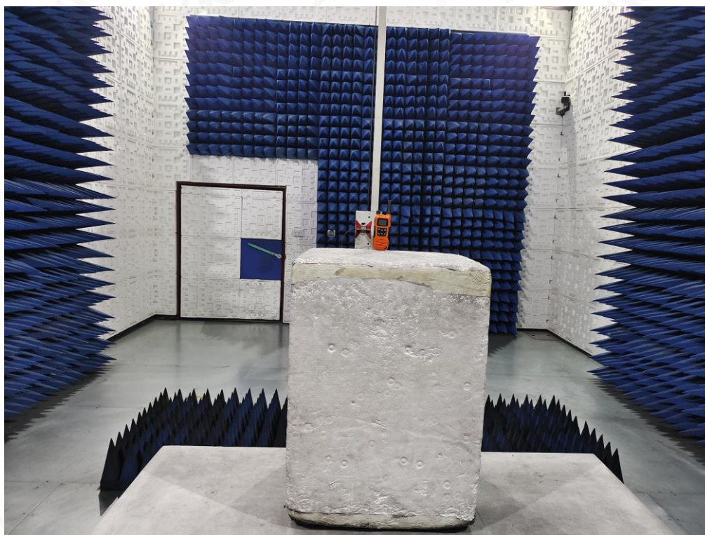
RADIATED EMISSION ABOVE 1G TEST SETUP
