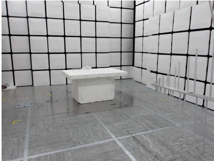
Photo 1.4-1 – Radiated Fundamental Field Strength Test Setup Photo [Front View]
