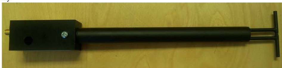
Figure 1 – MVG COMOSAR Validation Dipole
